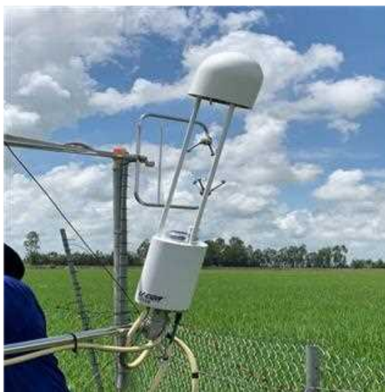
Figure 2.2: LI-7700 Device for Methane Emission Measurement in Rice Fields at Lang Sen Wetland Reserve, Long An.
