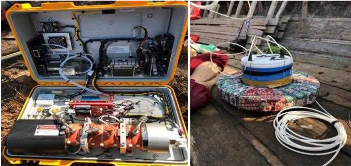
Figure 1.2. Left: Device picture of Ultra-Portable Gas Analyzer; Right: GHG emission measurement chamber
